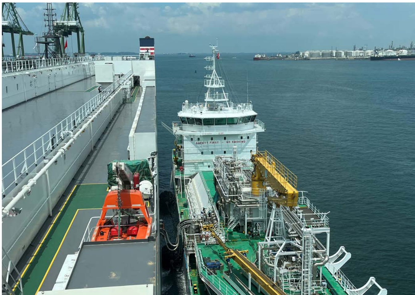
Simultaneous cargo operations and LNG bunkering on NYK's Jasmine Leader.
