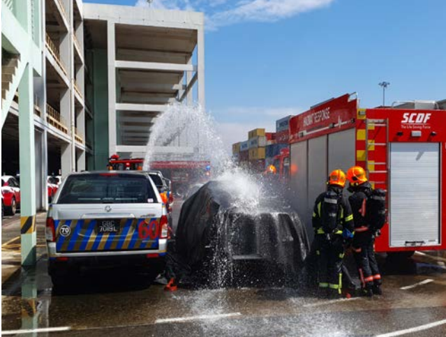
Fire blanket tested to cover affected EV completely.
